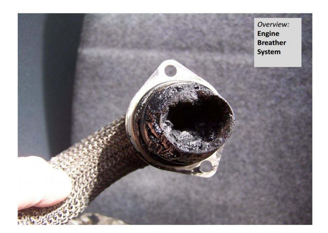
Overview of oil contamination, particle build up and oil path restrictions in the turbocharger leading to total failure of the turbocharger bearing system
